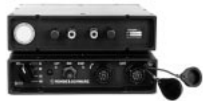
Remote Control and Rebroadcast Box GB3088 allows remote control of XV3088, ie traffic monitoring, ringing and transmitter keying from a field telephone using two-wire cable (Photo dr13-f1)
